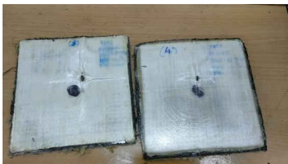
7733-10 layers with K49-CNT-22 layers after ballistics testing 7733 is in front
