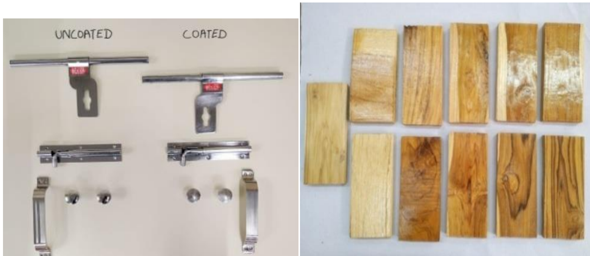
Fixtures and accessories (left ) and wood substrate (right ) coated with polymer nanocomposites based antimicrobial coatings
