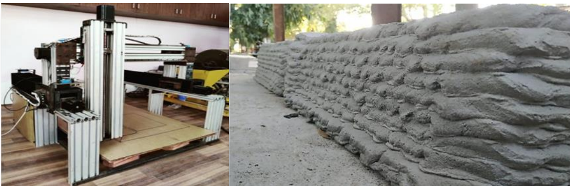
Photo 1: 3D concrete printer at CSIR-AMPRI Bhopal (left), 3D printed wall segment (right)
