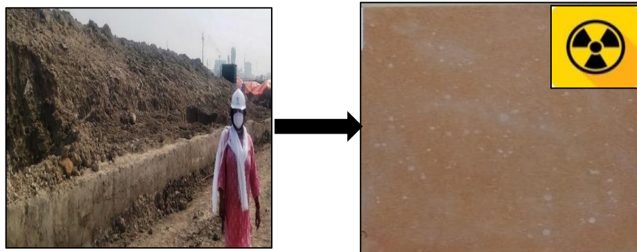
Brine Sludge - x-ray radiation shielding Tile
