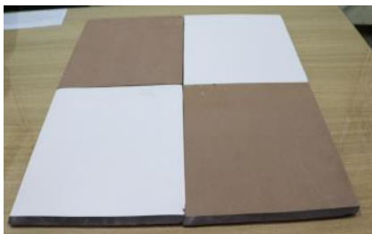
Joint free X-ray shielding tiles fabricated in pilot scale
