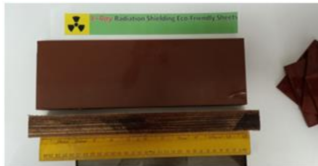
Figure 5: Lead free red mud based X-Ray radiation shielding panels
