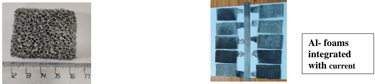
Figure 3: Open cell Aluminium foam plates developed at CSIR-AMPRI (85-90% porosity, Surface area: 10m 2 /gm)
