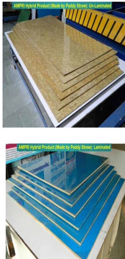
Figure 5. Unlaminated and Laminated and hybrid composite developed by paddy straw
