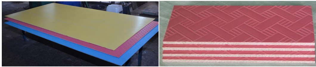
3 (a): Hybrid composite architectural cladding panels made from marble waste stream
