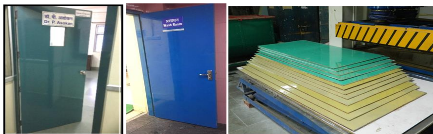
3(c) Hybrid sandwich composite Door and Door Frames made from marble waste
