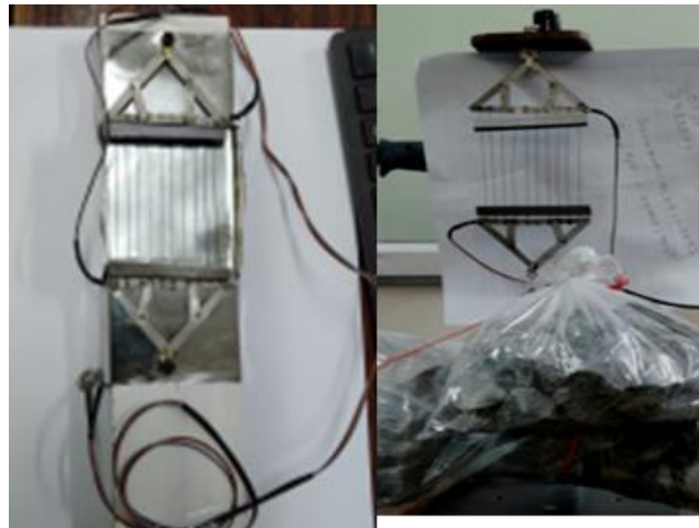
Figure. 1: SMA wire gage and its load testing
