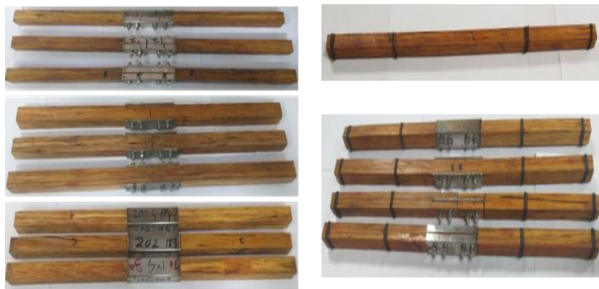
Figure 1 : Bamboo composite material with and without joints/ confinement
