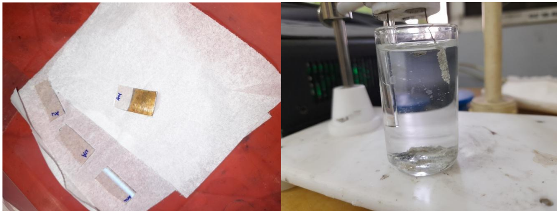
Electroplating of silver nanoparticle on ITO film and Gold nano particles on ITO film
