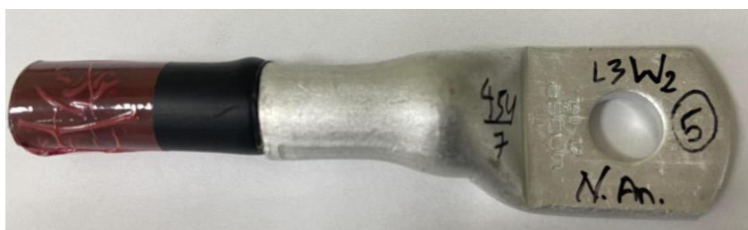
Figure 3. Electromagnetically crimped lug-cable sample
