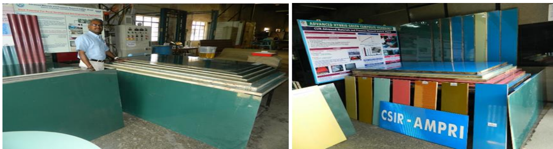
3(b): Hybrid green composites Board made from marble waste stream for furniture applications
