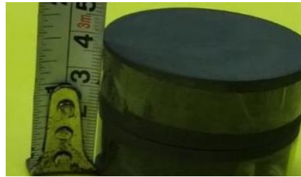
Figure 7 High density red mud blocks for industrial x- and \gamma -ray shielding:
