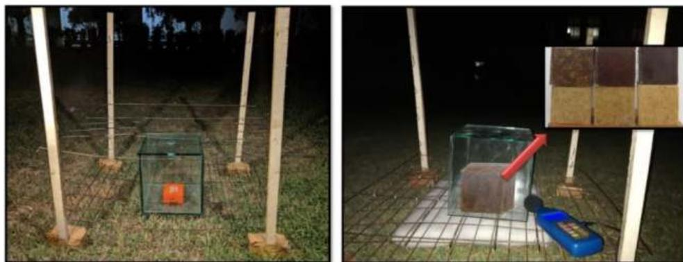
Fig.1 — Sound intensity measurement setup with (a) empty glass box and (b) composite samples.
