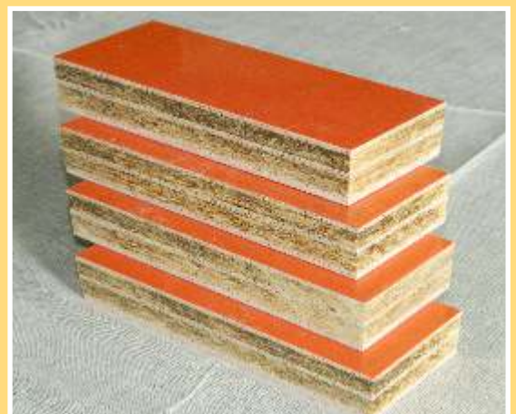
Sandwich composites made of wheat straw (30mm thickness)
