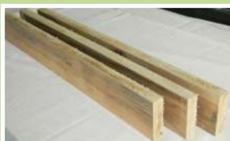
Parali particle boards : Flexural strength test specimens
