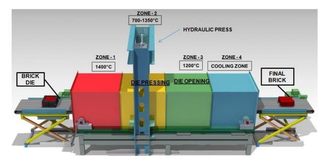
The schematic of semi-automated hot press, which is indent to build to make the joint free gamma and neutron shielding blocks.
