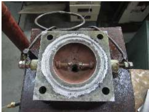
Hemispherical EHF die with Rogowski coil (to measure the pulsed current in the circuit)
