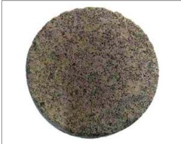
Ti-foam disc (size: 50 mm dia and 15 mm height )
