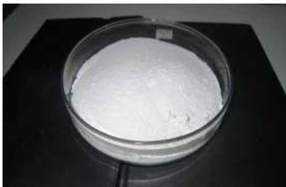
Synthesized nanoparticles of gamma alumina particles (Surface area: \sim 140 \text{ m}^2/\text{g} )
