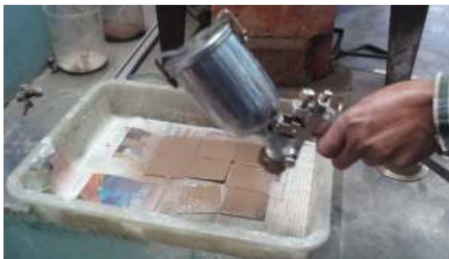
Phosphatic geopolymeric coating on mild steel by spray gun
