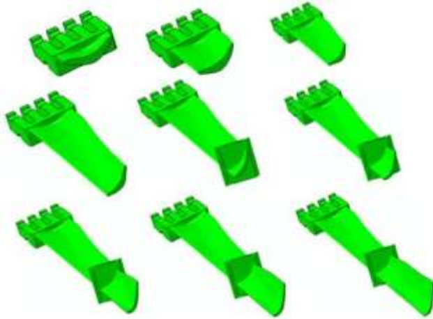
Solid models showing variation in the cross section of and profile rotation in the failed blade (no. 18)
