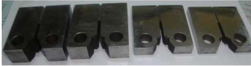
C(T) specimens of different thicknesses
