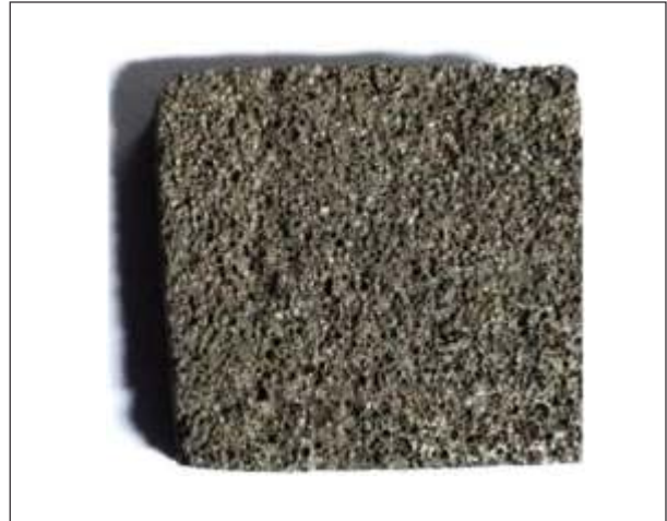
Stainless steel foam (size: 50 mm x 50 mm x 15 mm)
