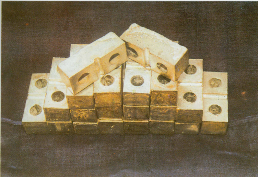
Squeeze cast half clamps supplied to BHEL, Bhopal
