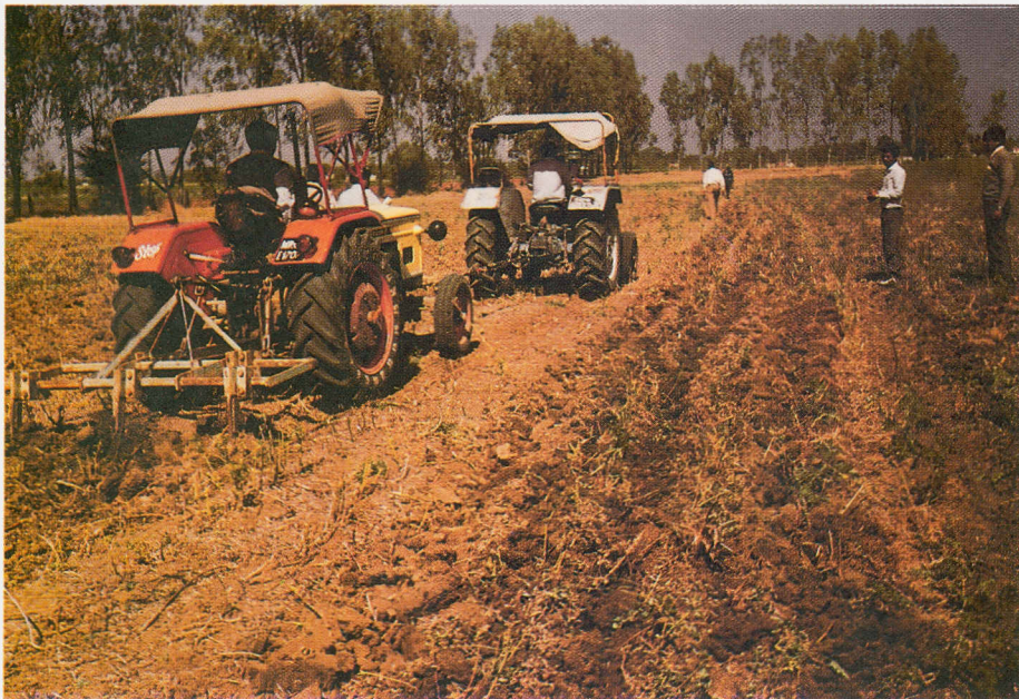
Drag force measurement of duck foot cultivator at CIAE, Bhopal
