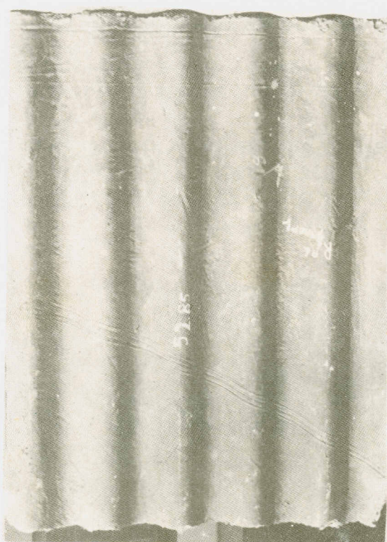
Fig. 12. Fibre (Sisal) cement corrugated roofing sheets.
