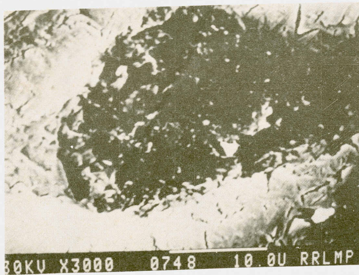
Fig. 6(b) Magnified SEM picture showing good bonding between particle and matrix.
