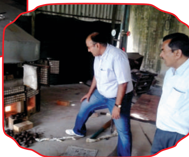
Sintering of red mud at semi pilot plant level with additives at CDGI, Firozabad for development of shielding aggregate
