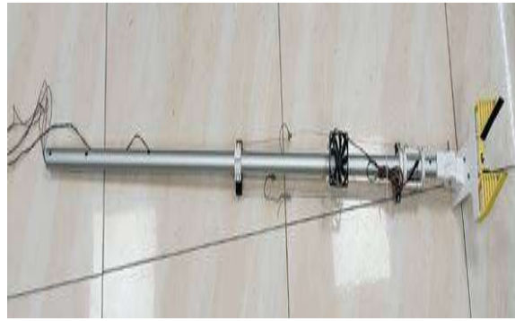
Preliminary prototype for SMA actuated soft gripper integrated with a part of assistive pole
