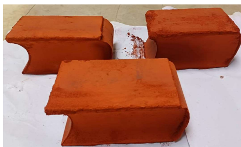
Interlockable gamma and neutron shielding bricks.
