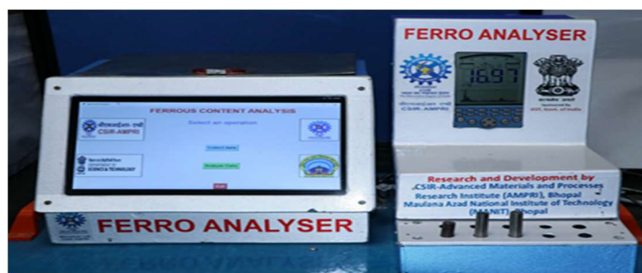
Ferro Analyser: Prototype instrument for ferromagnetic phase fraction analysis
