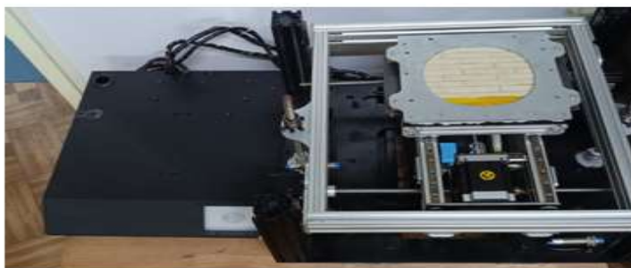
Fig: Customized motorized printing platform design
