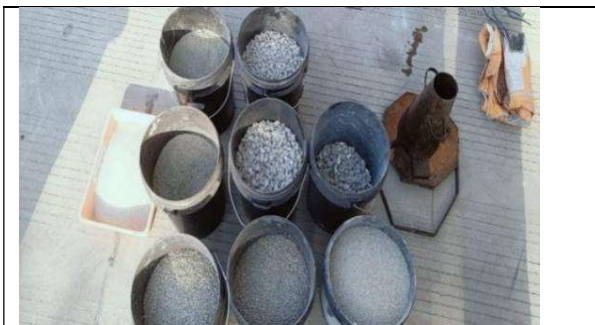
Different size fraction of broken sanitary ware aggregate
