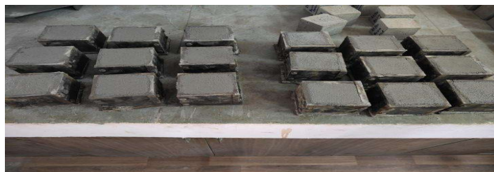
Casting of Mortar Cubes (70.6mm x 70.6 mm x 70.6 mm)
