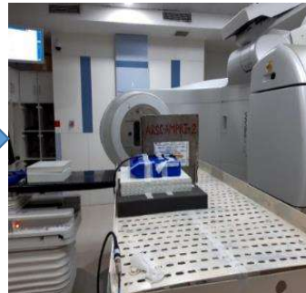
Radiation Attenuation Test before High Energy Linear Accelerator
