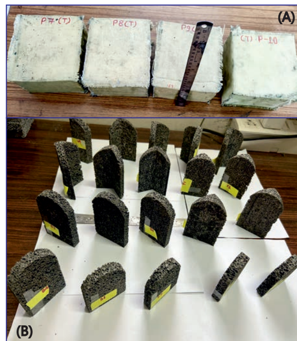
(A) Al hybrid composite foam core sandwich structures (B) Wire EDM machined Al hybrid composite foam structures to be assembled with BOOT-ANTIMINE prototypes for blast testing and evaluation
