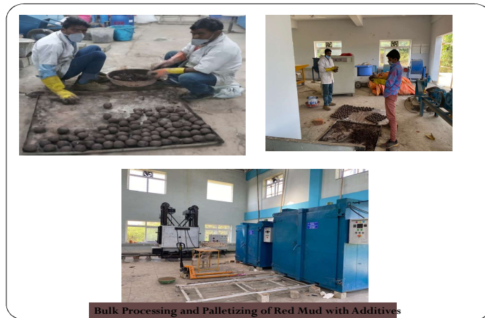
Bulk Processing and Palletizing of Red Mud with Additives
