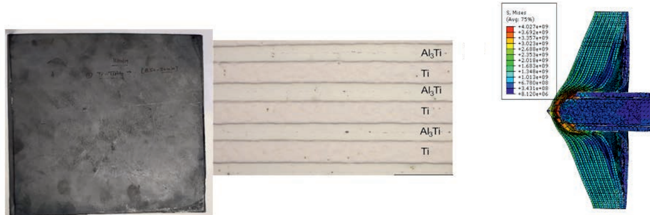
Figure 22 Schematic of Multilayer laminates and 8 mm armour plates (200mm* 200mm), Simulation of 8 mm Ti-TiAl 3 multi-layer plates with MSC NIJ III+ 7.62*39 mm Bullet
