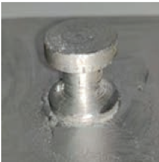
Figure 7 Evaluating bond strength of binder used in sandwich panel: (a) metallic bond; (b) pulloff adhesion tests performance of different binders used.
