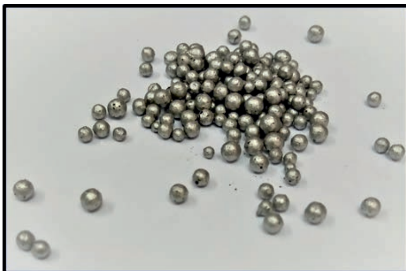
Figure 15 Prepared hollow sphere with different wall thicknesses.
