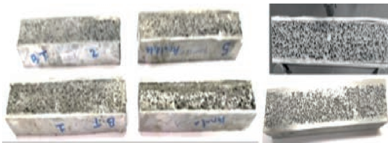
Figure 8 Flexural samples of metallic foam in-filled sandwich component.
