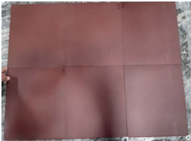
First batch of joint free X-ray shielding tiles fabricated by M/S Prism Johnson Ltd.
