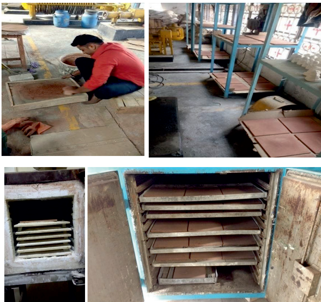
Fig. 15 Different steps of Tiles fabrication at semi pilot scale at Khurja.
