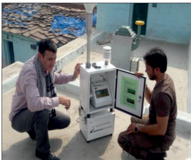
Installation of AAQM Equipment at identified Location
