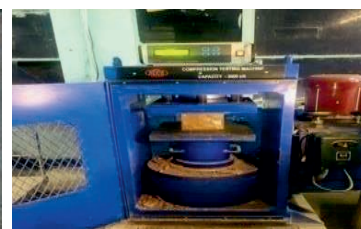
Evaluation of Compressive Strength of Red Mud-Fly Ash Geopolymer binder
