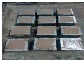
Cube Samples of Red Mud-Fly Ash Geopolymer binder
