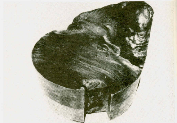
Fig. 16 Failure of coal mill shafts.
