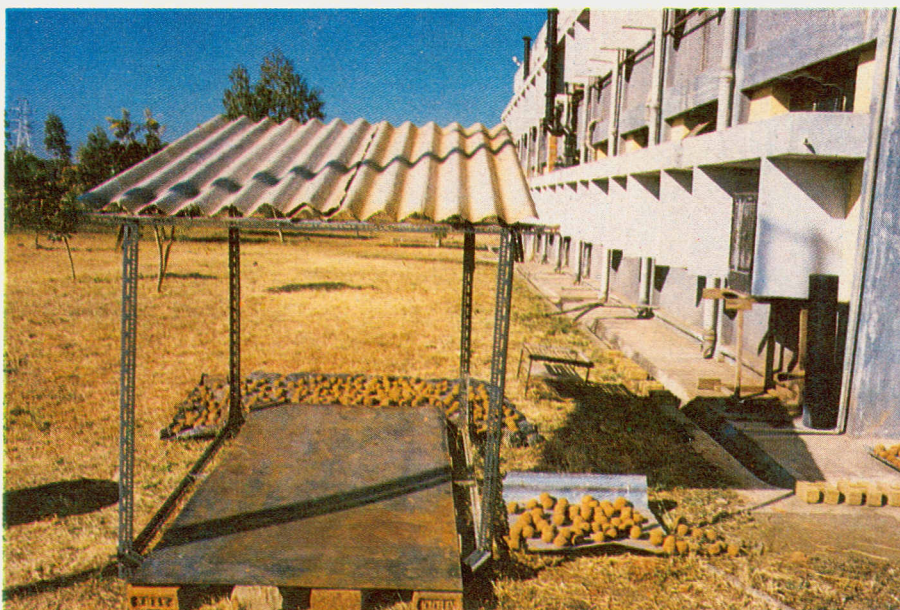
Fig. 7 Field weathering test of fibre-reinforced cement sheets.
