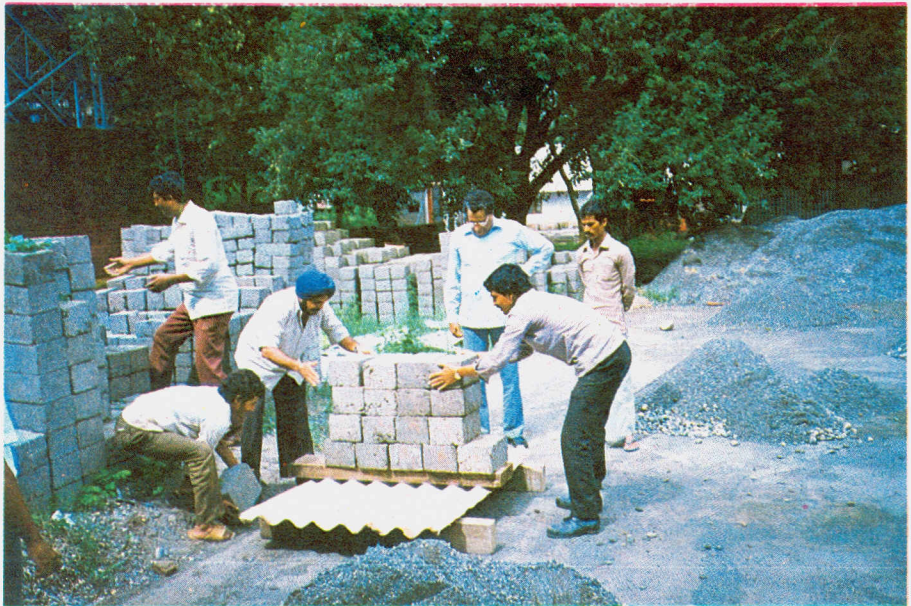
Fig. 5 Load testing of fibre-cement roofing sheets.
