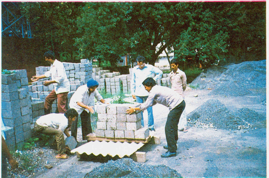
Fig. 5 Load testing of fibre-cement roofing sheets.
