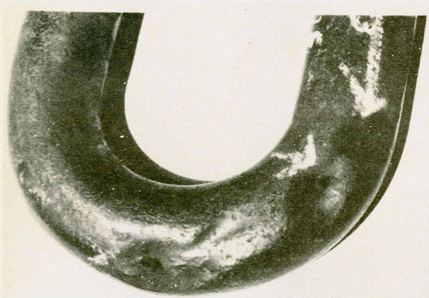
Fig. 22 Failure of boiler tubes on account of excessive erosion by the impactation of abrasives in flyash.
