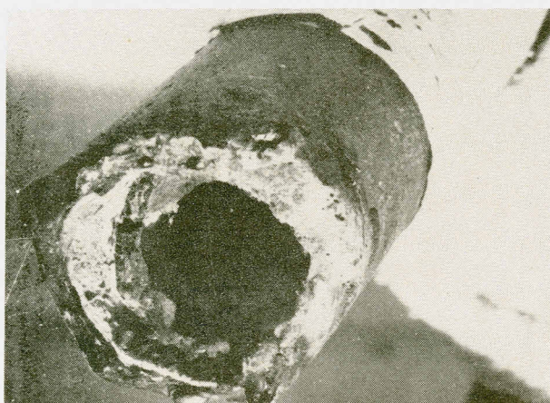
Fig. 20 Failure of water wall tubes on account of poor water chemistry resulting in deposits on the inner surface of the tubes.
