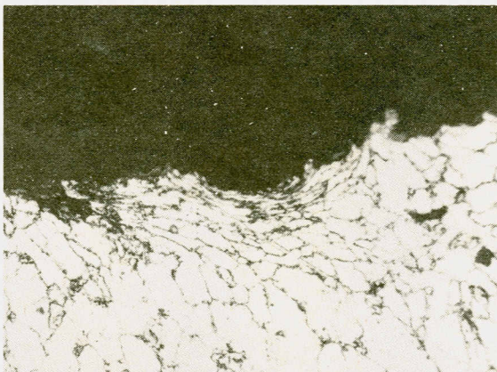
Fig. 22 Failure of boiler tubes on account of excessive erosion by the impactation of abrasives in flyash.
