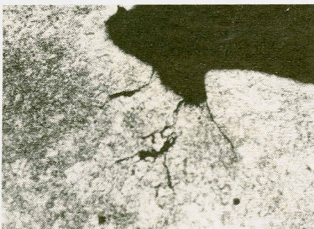
Fig. 17 Failure of blades on account of stress corrosion cracks.
