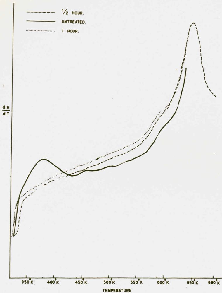
Fig. 17: Typical dH/dt vs. Temp. plot for Sisal
