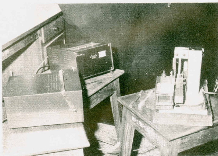
Fig. 4: Set up for measuring, damping capacity of composites at RRL, Bhopal.
