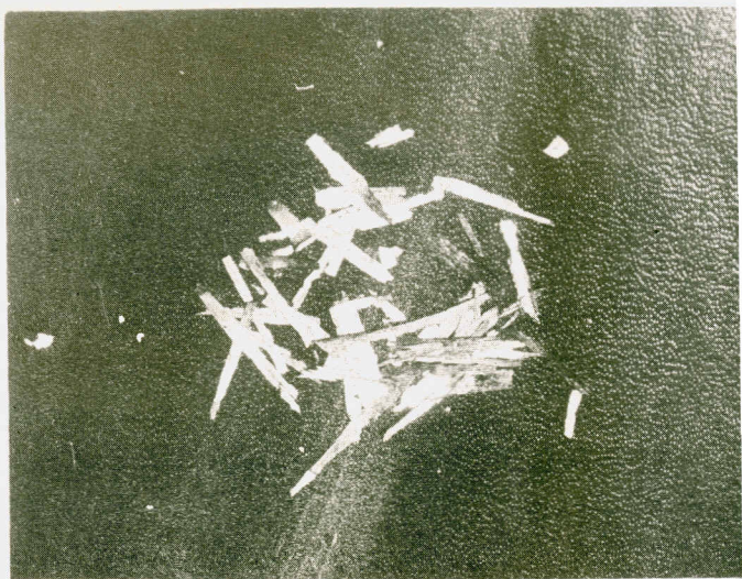
Fig. 7 : Discontinuous ribbons of Al-graphite composite material.
