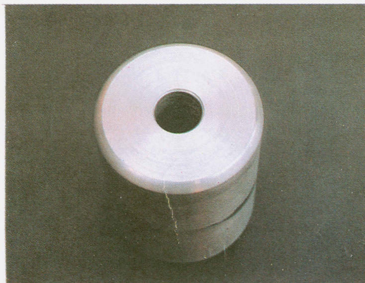
SiC whisker reinforced 2014 aluminium alloy matrix composite billets produced from ingots ready for extrusion
