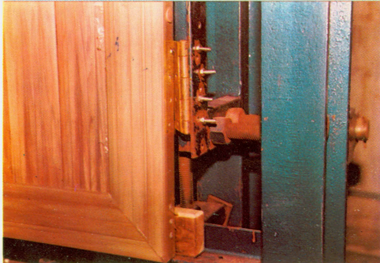
Misuse test performed on a door
