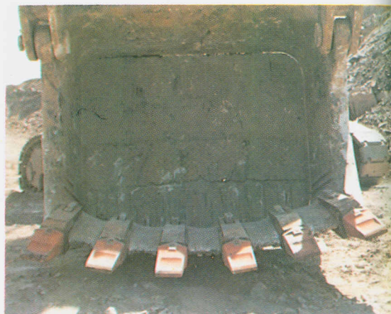
Excavator bucket fitted with shovel teeth supplied by RRL
