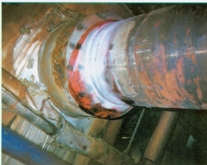
In-situ dye penetration test
