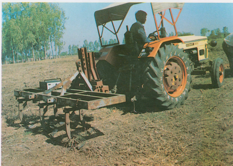
Sweeps made by RRL under field tests
