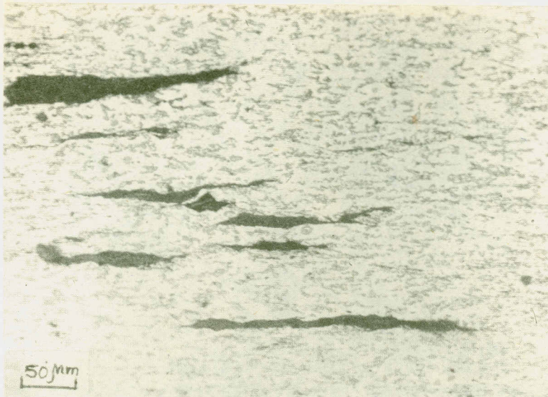
Fig. 5. Typical microstructure of LM 13-3 wt.% graphite hot rolled to 67% reduction (Photograph taken at the long transverse direction).
