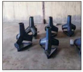
Geopolymeric Tetrapods in Moulds developed by CSIR-AMPRI, Bhopal
