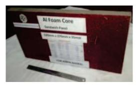
Giant Aluminium foam billet and foam core sandwich panel
