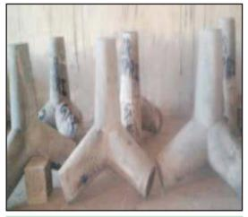
Finished and Properly Coded Geopolymeric Tetrapods at NTPC Simhadri
