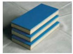
Sandwich composite made out of Marble wastes for possible application in partition wall
