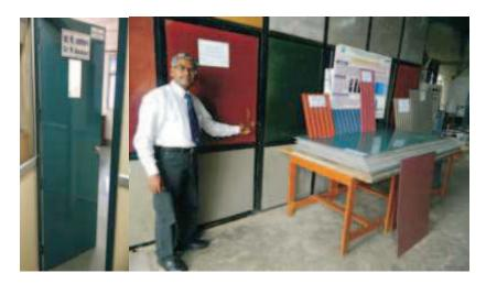
Advanced Hybrid Composite Wood and Wood Substitute Materials (AC- Wood) developed at CSIR-AMPRI Bhopal and have been demonstrated for use as floor tiles, door, partition panels, false ceiling
