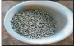
Fine aggregates (sand sized) prepared by fly ash
