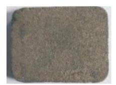
SS-foam blocks with 80% porosity (pore size 250 micron)
