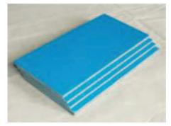
Panels made out of Marble wastes for possible application in wall tiles and floor tiles
