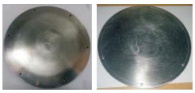
Fig. 2 Wear Test Sample plates: (a) Cast Iron; (b) Developed ALMMC
