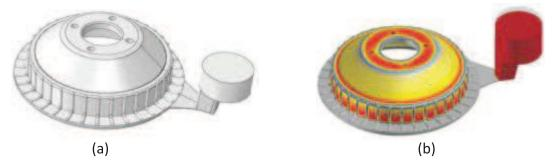
Fig.1 Casting Simulation of Brake Drum Component: (a) Solid Model; (b) Solidification Results
