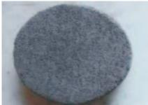
SS-foam disc filter (pore size 50 micron)
