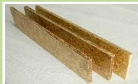
Parali particle boards : Flexural strength test specimens
