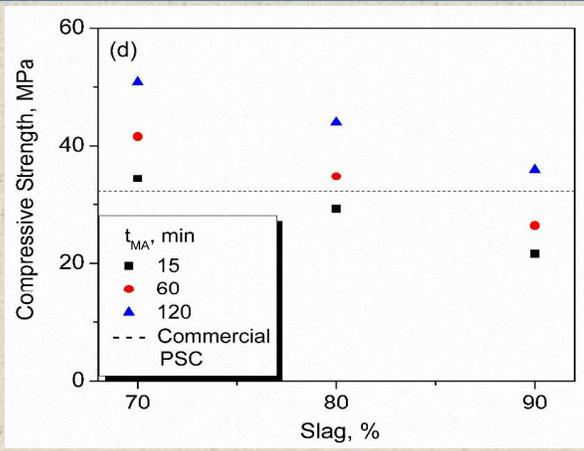
*Vibratory milled slag for 15, 60 and 120 min mixed in various proportions with clinker*
