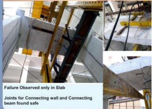
Failure Observed only in Slab
