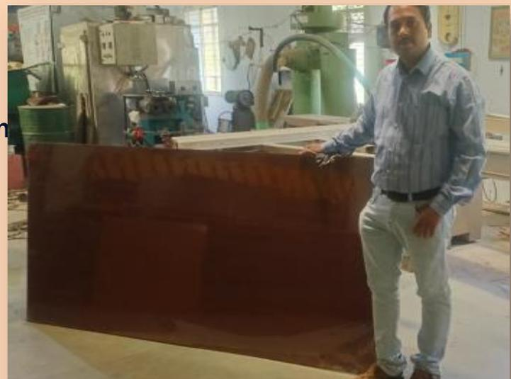
Full Scale X-Ray Radiation Shielding Panel 12 mm Thick
