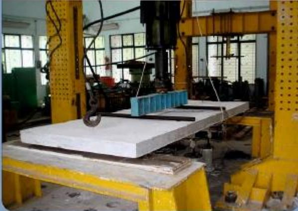
Development of Precast lightweight Concrete Sandwich Roof Panel using EPS
