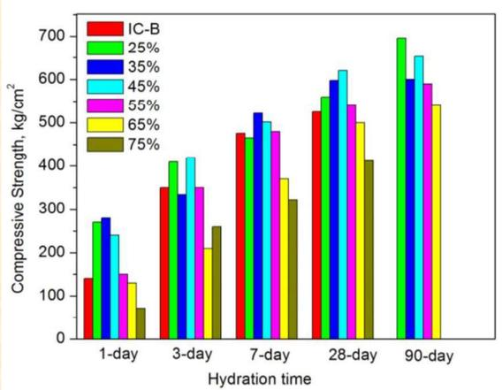
*With mechanical activation of fly ash, incorporation of fly ash up to 65% is possible*
