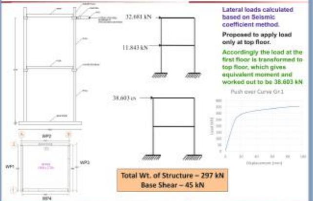
Lateral loads calculated based on Seismic coefficient method.
