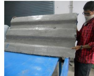
Production of TRC roofing sheet using TRCPT
