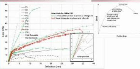
Load Deflection Curves of CSPs follow tri-linear relationship up to the Ultimate Load similar to Ferro-cement Panels under Bending
