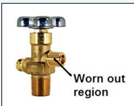
(a) Contact finger for contactors (b) Nozzle of commercial gas cylinder value and (c) Lug-cable crimp
